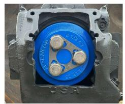
"Clinchfield 100" office car (WATX 100): at the Spring St. Coach Yard receiving upgrades. At left we see new roller bearings recently installed recently at NCTM in Spencer, NC.
