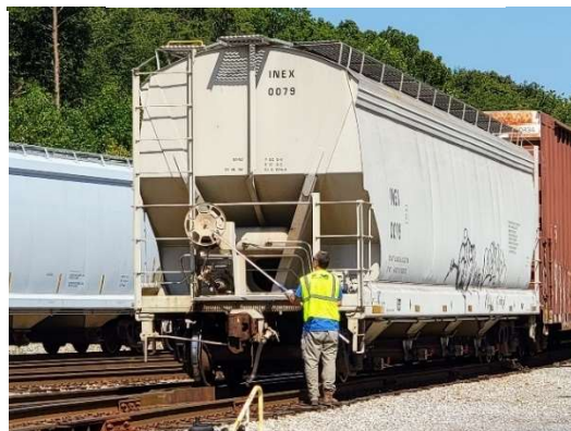
[Below] Conductor setting a Covered Hopper's brake preparing it for car kicking.
