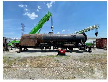
removed one at a time. Each driver wheel was dragged using a telehandler rather than rolled due to the lack of side rods acting as a balance to the counterweights. The engine was then lowered onto four steel pedestals. The driver wheels will be sent to the Tennessee Valley Railroad Museum in Chattanooga where they have the special machinery needed and FMW Solutions will perform the repairs and needed maintenance.
