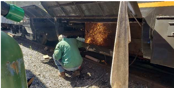
[Left] Mike Dowdy cutting out the old hot water compartment; [right] Mike and Art Devoe working on Perkins Genset.
