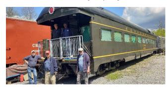
"Clinchfield 100" office car (WATX 100): a new platform railing has been installed, making it safer for passengers to ride on the platform. Leading the effort were Mike Dowdy and Gary Lombardi.
