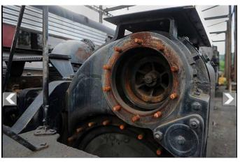
Front engine left-hand piston valve. [Baltimore Sun] well over its few years of service, and it had been "rode hard and put away wet," to borrow an equestrian term. It was going to be a somewhat bigger project than first imagined. The new tube sheet will go in shortly, and new tubes and flues on the property,
