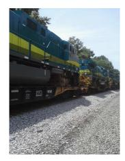
[ ] A shipment of new VALE BB-40-9W diesel locomotives are seen passing through Appomattox, VA on their way to Norfolk, where they will be loaded onto a ship bound for Brazil. These units are an odd 5' 3" gauge used exclusively in the nickel and iron ore mines served by the Valley Railroad Company located in Brazil. The trucks for these units are loaded on separate flatcars.
